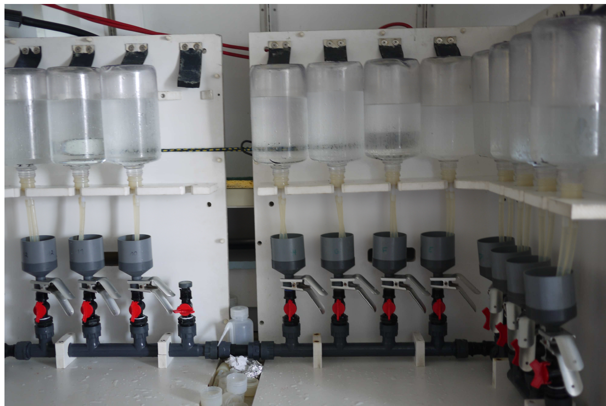
Water filtrations in the wet lab of the R/V Téthys II , on samples taken from a CTD cast. The filters are subsequently used for quantification of phytoplankton pigments (HPLC) and particulate absorption.
